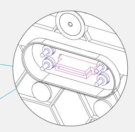
Using custom connectors, to ensure the safety of high-current transmission and signal transmission stability, which is completely different from the traditional row pin and female connector.
